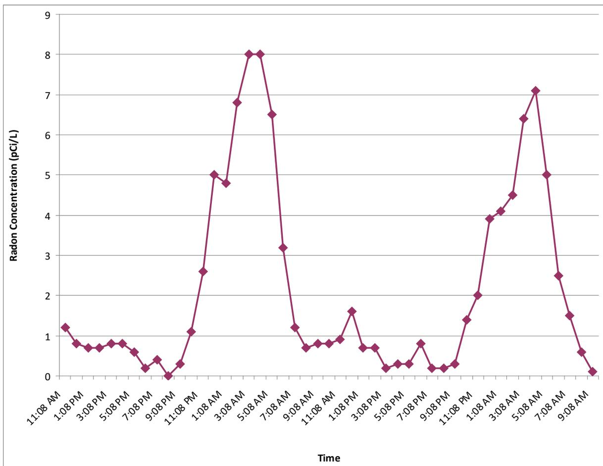
*Note on Graph: Measurements were made in a student nutrition classroom (aka 'home-ec') using a CRM. A year prior, a 10-month test showed radon levels of 5.0 pCi/L. The results shown in the graph were from testing conducted in February.*
