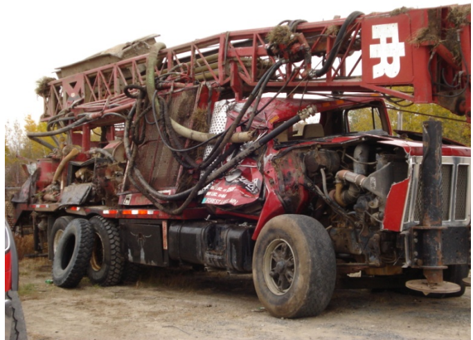
McCullough and Sons, Inc. Ingersoll-Rand TH-55 rotary drilling rig after crashing due to blown tire.
