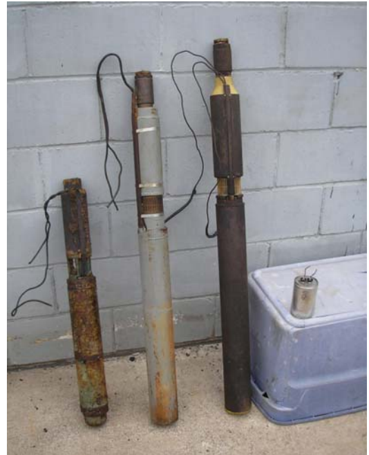
Two-wire submersible pumps containing capacitors filled with PCB dielectric fluid.
