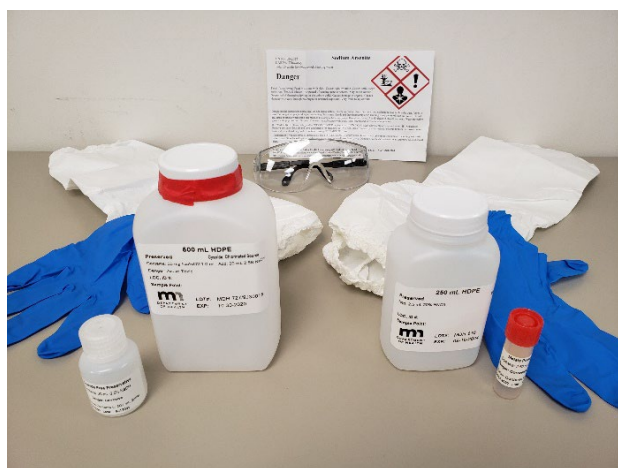
Left: 500 mL Bottle with 1.0 mL of 50 mg/mL Sodium Arsenite (NaAsO 2 ) and Sodium Hydroxide (NaOH) Preservative
