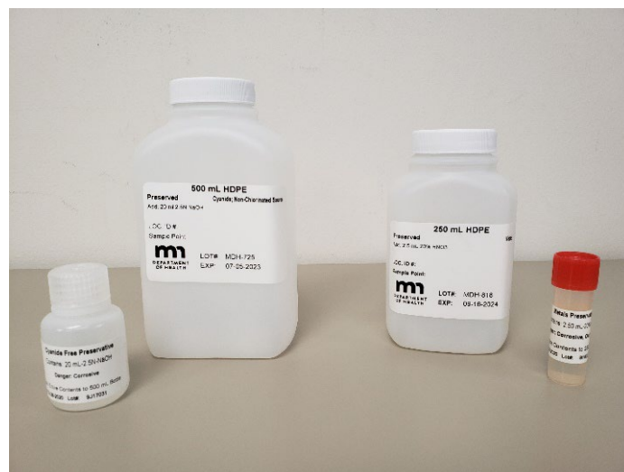
Left: 500 mL Bottle and Sodium Hydroxide (NaOH) Preservative
