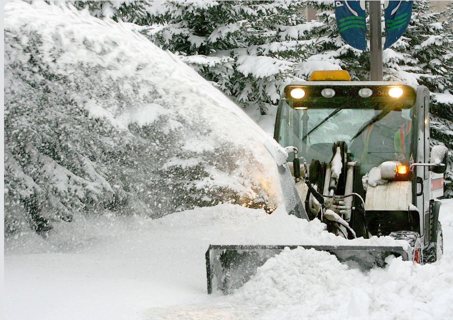
Figure 7: A City of Duluth employee clears a sidewalk with a Bobcat tractor. Sidewalk snow clearing crews follow street plows to reduce snow that is pushed back and forth between facilities. Credit: Duluth News Tribune
