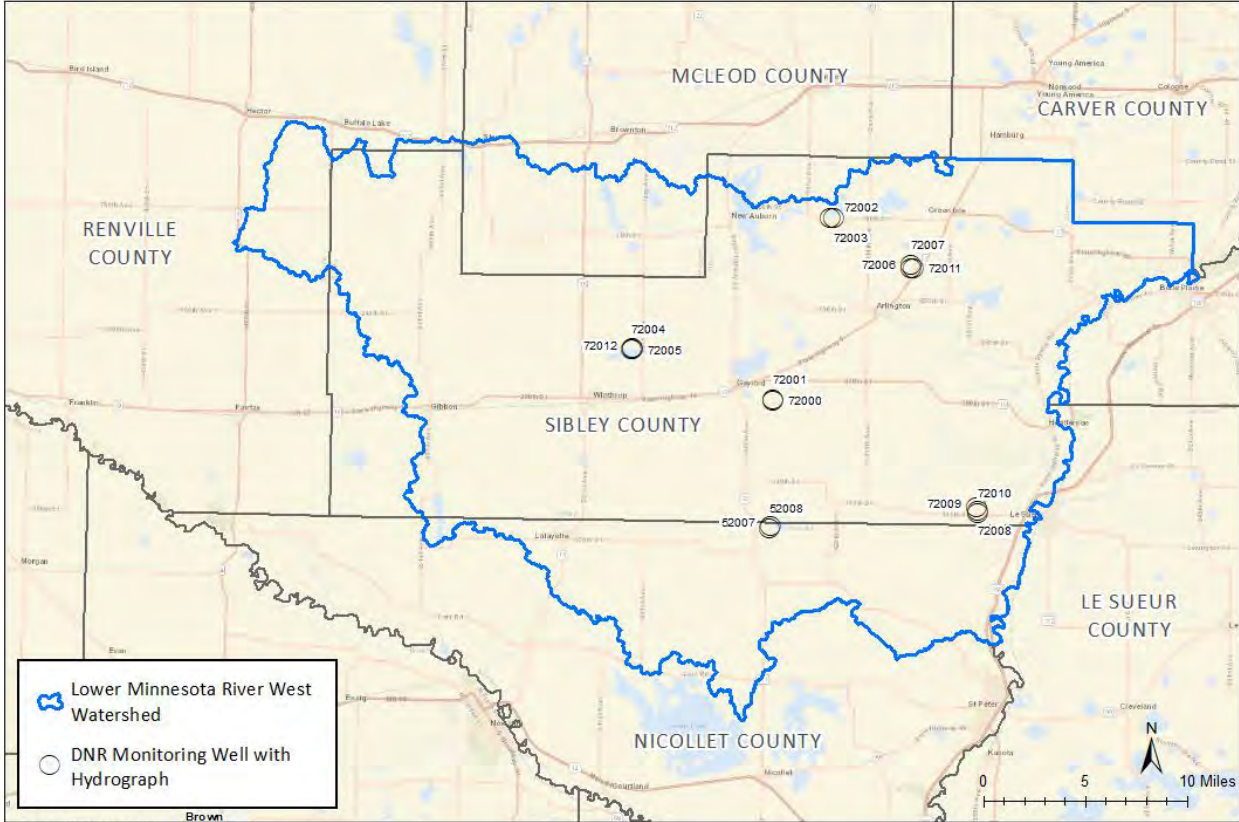
Figure 24: Location of active groundwater-level monitoring wells with hydrographs. No groundwater-level monitoring wells had sufficient length of record of water-level data to calculate a long-term trend, which requires a minimum of 20 continuous years of data.
