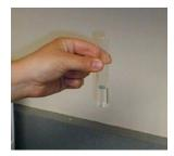
3. Add the tablet, powder, or drops needed for the desired chlorine measurement (free or total) to the sample vial. Be sure not to touch the reagent. Cap the vial and gently invert or swirl to mix in reagent. Avoid excessive shaking of the vial which could create air bubbles and influence the measurement.
