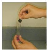
4. Allow color to develop according to your kit's specific instructions. Then place sample vial into comparator or digital colorimeter.
