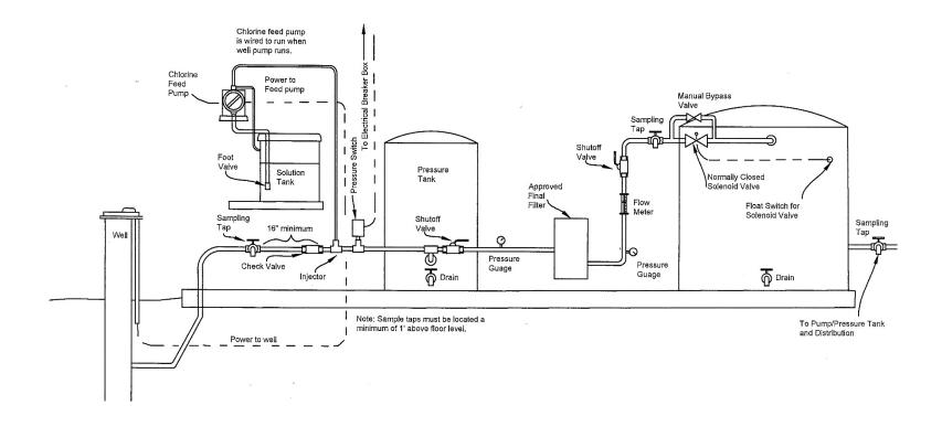
Water is pumped from a well and is treated with chlorine before flowing through filtration and storage. The final filter is rated for the removal of microorganisms. Storage allows for contact time before re-pressurization and service to the distribution system.
