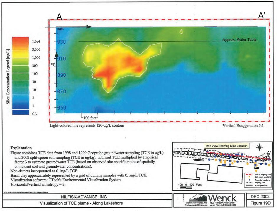
Figure 6: Cross-section of TCE Plume Illustrating Higher Concentrations at Depth
