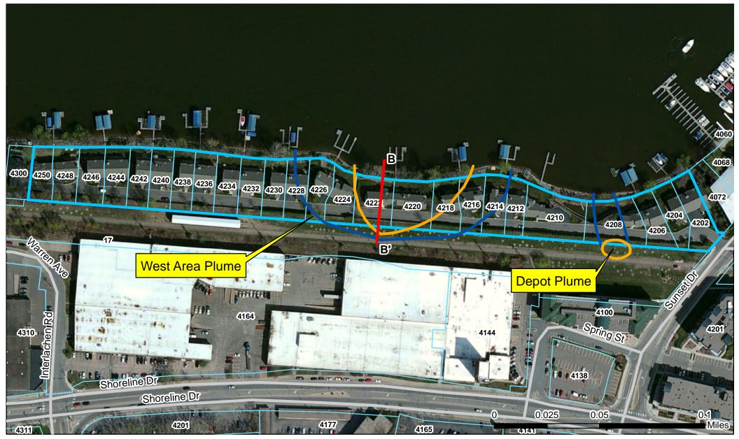
Figure 3 - Current Site Map With Groundwater TCE Concentration Contours
